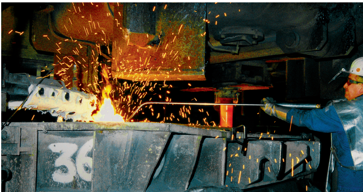
Bath temperature measurement in the tundish
